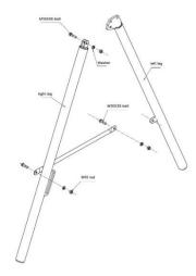
2. Connect the two sets of support legs assembly and one set of shooting target bracket with M10x15 bolts, nuts and washers).
