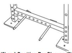
7. Add your Spotting Bars (6) and Spotting Bar Sleeves (8): Choose your preferred location for the Spotting Bars (6). Push 1 Spotting Bar (6) slightly (about 0.5") through your preferred hole on the Main Frame (1), then hold the Spotting Bar Sleeve (8) in place so that you can push the Spotting Bar (6) through the Spotting Bar Sleeve (8) and finally through the hole on the other side of the Main Frame (1).
