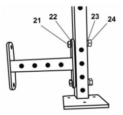
Repeat this process for all 4 bolts on one side, then proceed to the second *Extension Upright (17)* and again attach side bracings to the OUTSIDE.
