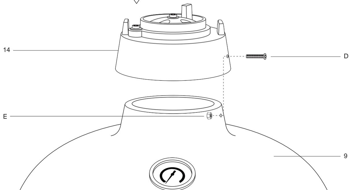
**STEP 11** - To attach the top vent (14) to the Kamado Grill (9) place it on top and align both the bolt holes. Secure using 2x bolts (D) and nuts (E). Ensure that the top vent bolt is on the left hand side when assembling it.
