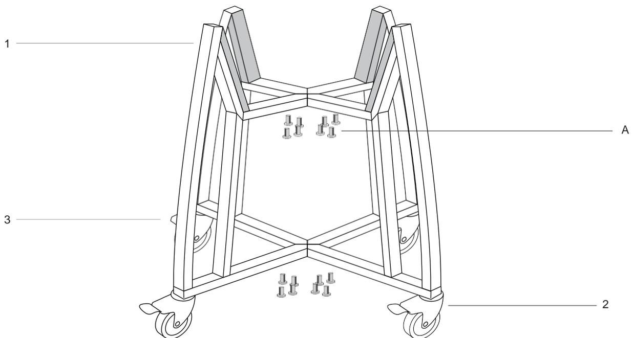
**STEP 4** - Secure the brackets (1) to the cross pieces (4) by using the 16x screws (A). Make sure the cart is secure and all of the screws are tight before placing the Kamado Grill (9) into it.
