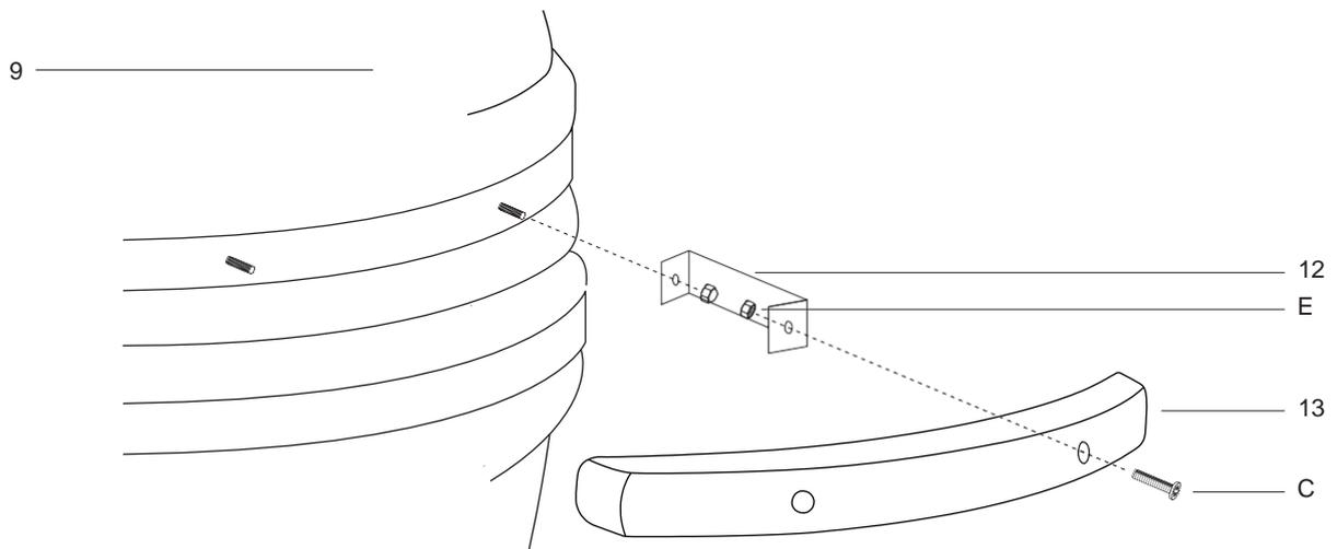
**STEP 10** - To attach the handle (13) to the lid of the Kamado Grill (9) start by attaching 2x handle brackets (12) using the 2x pre-attached bolts and dome headed nuts. Attach the handle (13) to the brackets (12) using 2x bolts (C) and nuts (E).
