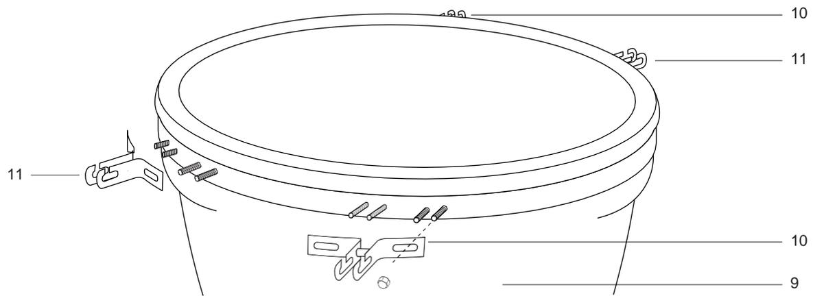
**STEP 12** - Attach the 2x table brackets R (10) to the Kamado Grill (9) using the 4x pre-attached bolts and dome headed nuts per bracket. Please note the position shown in the above diagram.
