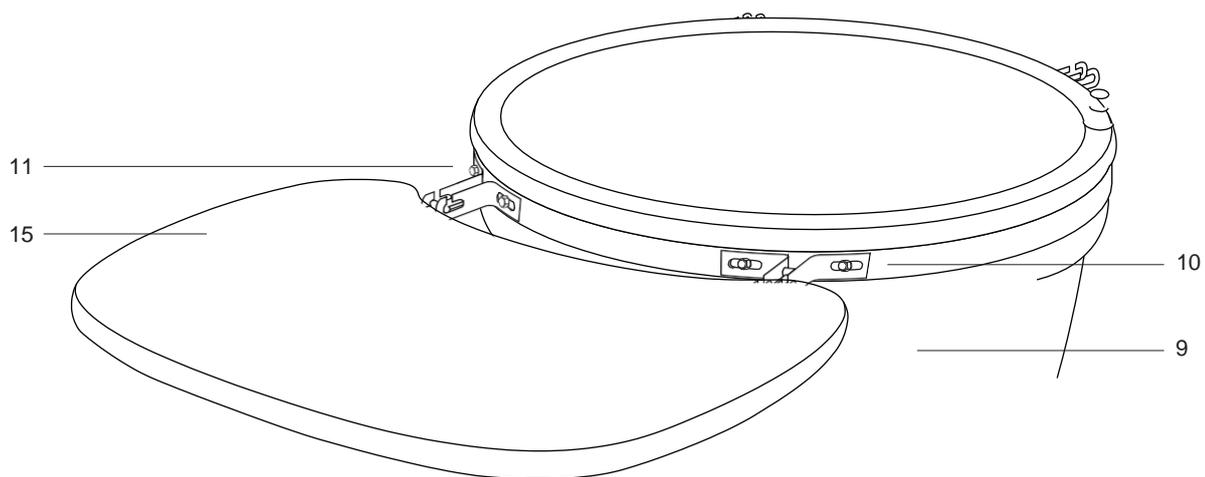
**STEP 14** - Insert the 2x table hinge (15) into each of the table brackets (10 & 11).
