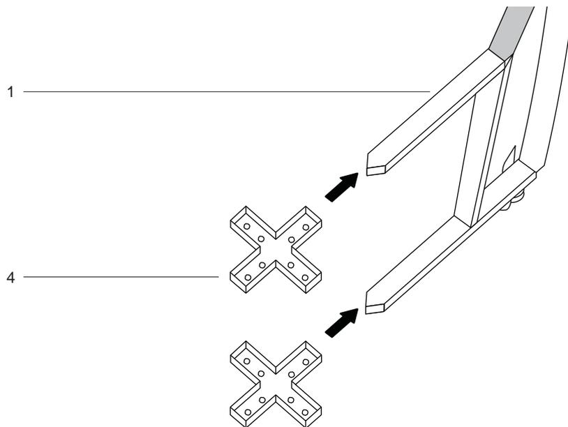
**STEP 2** - To assemble the cart insert the two cross pieces (4) into one of the four brackets (1) from both the top and bottom.
