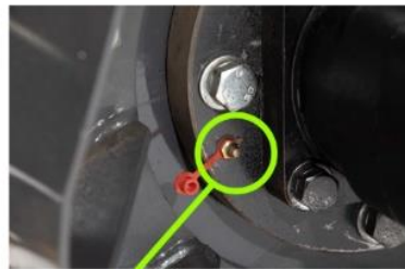
Motor Grease Point
