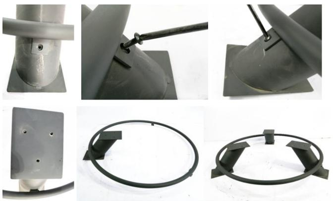
STEP 3 Assemble fire bowl with legs and align holes. Insert bolt M8x15 and tighten with a screwdriver. Same for all legs.
