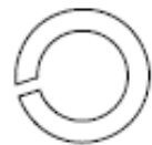
No. 36 \phi 10 Spring Washer (1)
