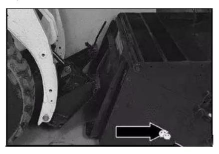
Ensure that the lever of quick-change mechanism does not collide with the sweeper.
