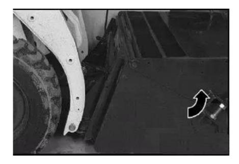
• Turn the engine off and leave the cab. Depress the quick-change lever until the locking pin is fully inserted into the pin hole in the mounting bracket to be locked (Figure below).
